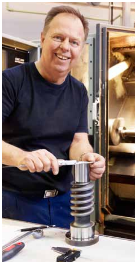
The precision of a worm gear is examined before production starts at Mikroverktug.
