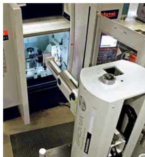
Automated machining cell with robot at Resinit.
