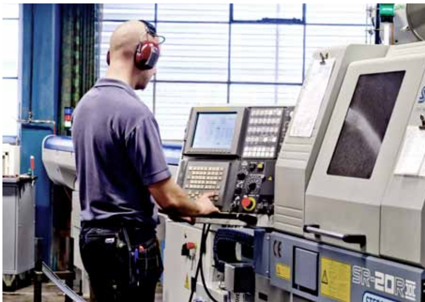
CNC-controlled lathe adapted for machining long components.
