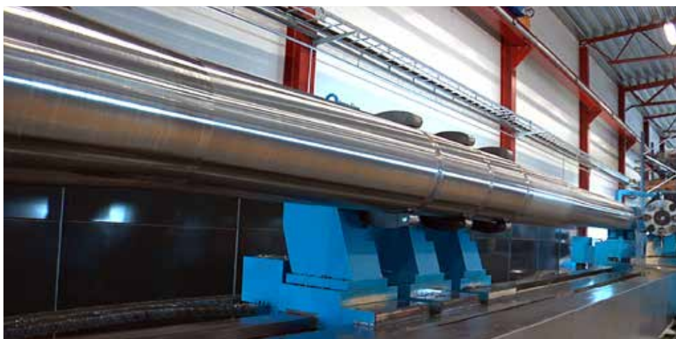
Machining a propeller shaft weighing 15 tonnes at KMV.
