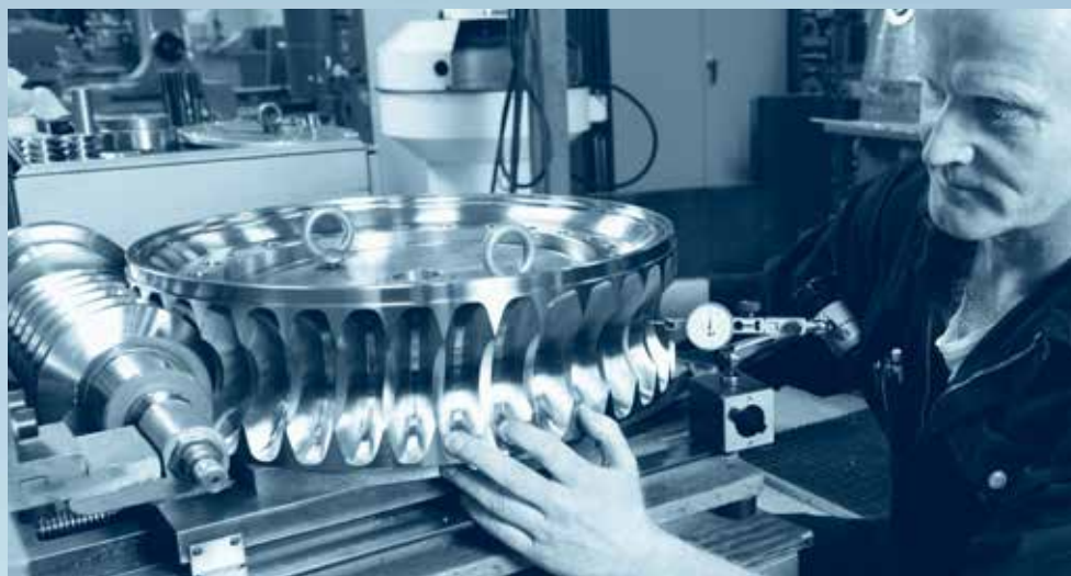
Verification of tooth data for toothed gears at Mikroverktøy, where each thousandth of a millimetre makes a difference.
