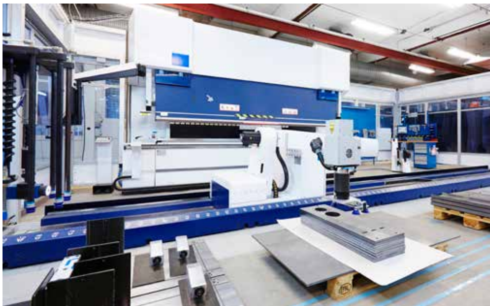
Production in fully automated machining cell for bending at Fredriksons.
