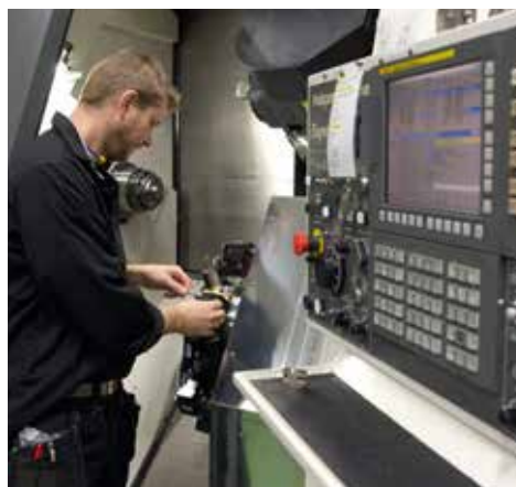
Rigging for new item in multi-operation lathe at LK Precision.
