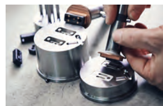
Tool insert adapted for small plastic components in short production runs.
