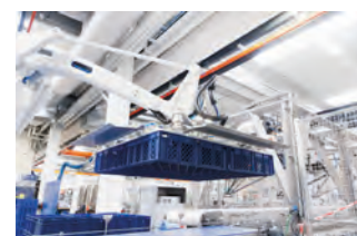
Automated handling equipment for bag packaging.
