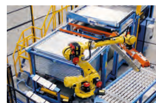
Accumulation and distribution solution for lid handling.
