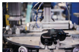
Machining cell for steering servo container made of polyamide.
