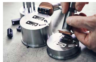
Tool insert suitable for small plastic components in short production runs.
