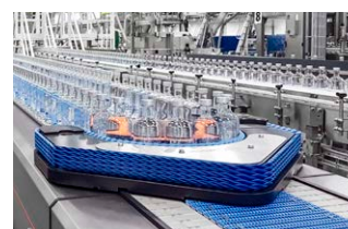
Buffer solution for glass bottles that regulates the flows in production lines.
