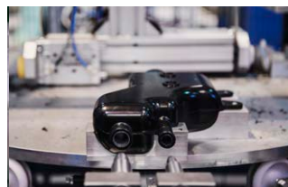
Machining cell for steering servo container made of polyamide.
