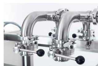
Pipes and drain valves with high hygienic demands for bioprocesses.
